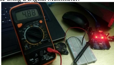
Figure 8. Voltage measurement on buzzer
