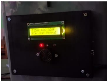
Figure 10. Warning via LCD, LED light and buzzer
